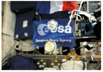
Shown here aboard the ISS, Aquapad is a new device for testing water quality on the station.
